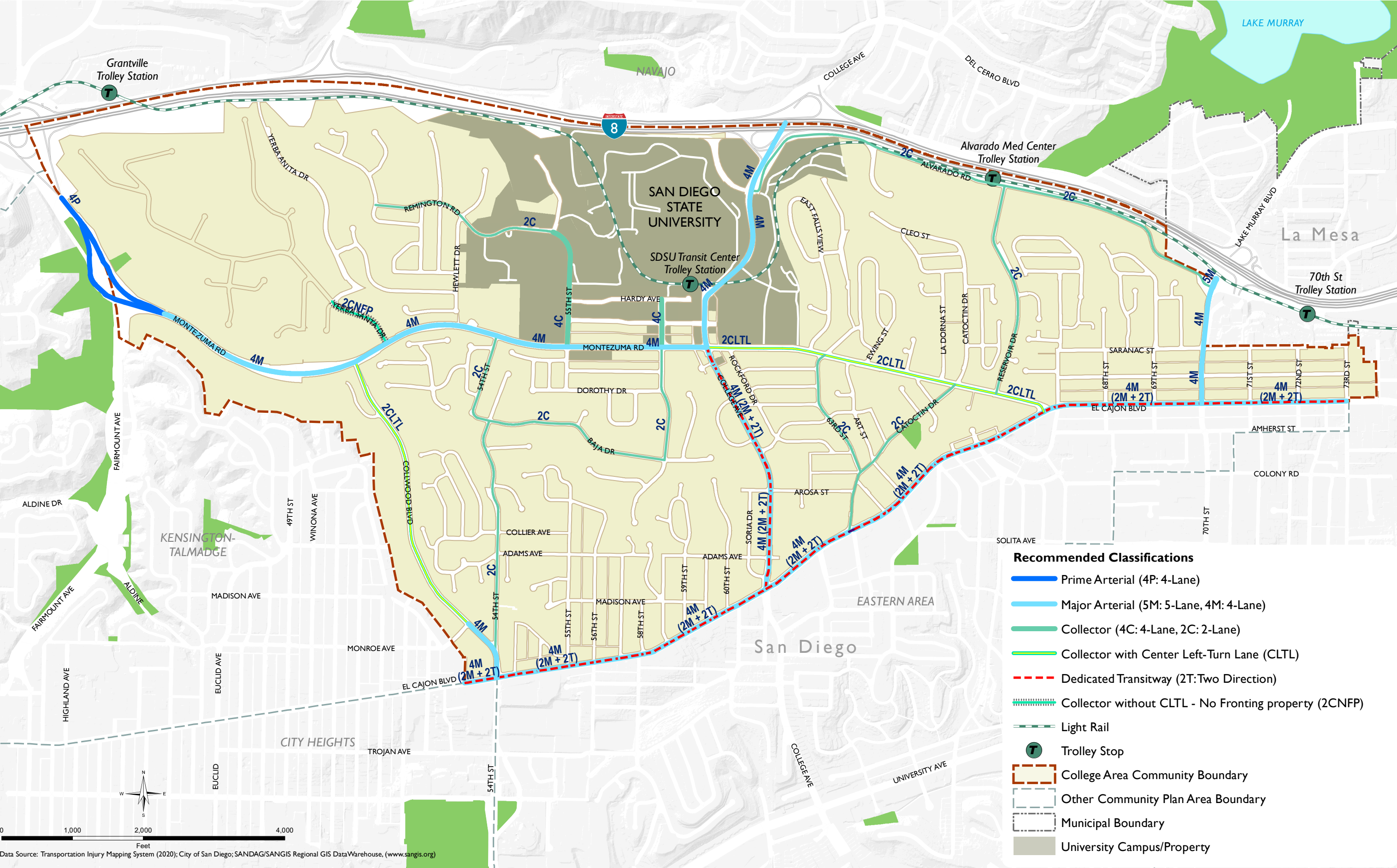
Figure 3: Recommended Roadway Network Classifications
