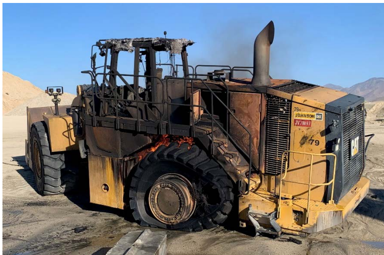
Left rear of loader just prior to full extinguishment.
