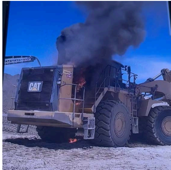
Fire in engine compartment
