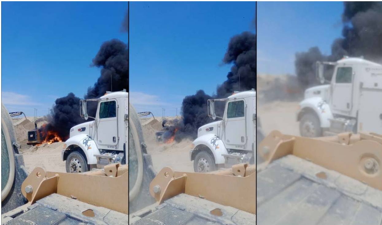
Right-rear tire explosion prior to FD arrival. The windshield of the white truck was broken during the blast.
